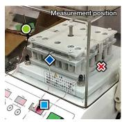
The 48 pcs-holder for 2 mL tube TH-0248T with 48 tubes and Metal crusher that was frozen with liquid nitrogen was attached to the unit. Then, the temperature change of each part while shaking at 1200 r/min was measured. The cryogenic temp. was completely kept for 30 to 60 sec which was required for crushing. The display temp. indicates the temp. stage of the top surface on which the holder is placed.
