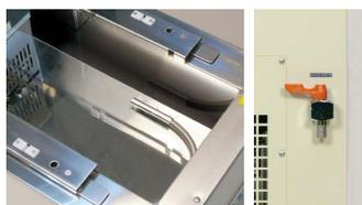
Personal Lt-10F is equipped with a drain hole as the water bath inside it cannot be removed due to its construction (Water bath inside Personal Lt-10F and Drain cock on the back are shown in left figure). Water bath inside Personal H-10 can be removed.
