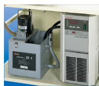
Combined with Circulator for Open circuit
