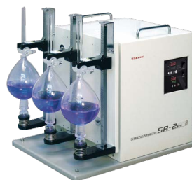
Shaking rack for separating funnel (1L x 3) (HE-3 shaking table for SR-2) Example of application (Container not included)
