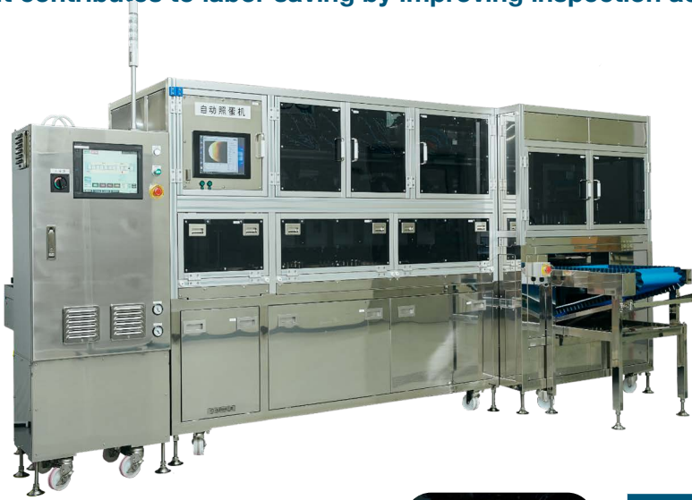
It removes the underdeveloped eggs by capturing the inside of fertilized eggs by CCD cameras. Available to inspect up to 32,000 eggs per hour.
