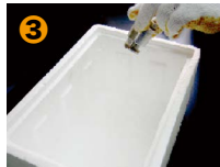
3 Soak and freeze in liquid nitrogen until bubbling stops.
