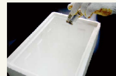
Freeze the whole holder with excellent cold insulation using liquid nitrogen
