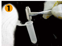
1 Put the specified amount (below) of sample and metal crusher into the vessel.
