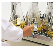
Two-tier platform shaker NR-150N with Clamps (optional)
