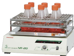
NR-20 with Optional shaking platform
