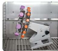
The rotator has a safety function to stop the rotation when it cannot keep itself horizontal.
