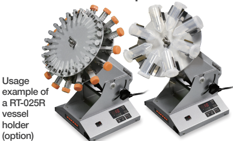
You can fix the angle freely between 0° and 90°.
