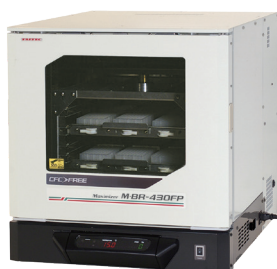
MBR-430FP with the Optional Shaking platform for Deep well plates
